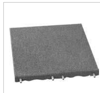
Rubber Tile 8048506 30mm. Critical Fall height \leq 1.0 8048509 50mm. Critical Fall height \leq 1.5 8048512 80mm. Critical Fall height \leq 2.4 8048515 90mm. Critical Fall height \leq 3.0
